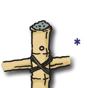
\* 把竹棚的竹端鑽穿或用幼沙填塞。 Fill up ends of bamboo scaffoldings with sand or drill them with holes.
