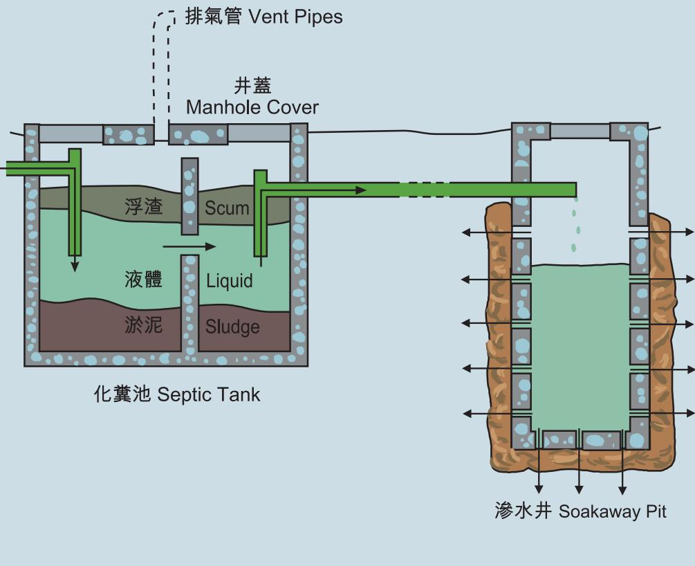
若化糞池的設計及保養不完善，蚊子便可 在池內的液體滋生。要防止蚊子在化糞池內滋生，便要最少每三個月進行定期檢查一次，以確保：The liquid in the tank can provide a breeding place for mosquitoes if the tank has not been properly designed and maintained. To prevent mosquito breeding in the tank, one should inspect the tank at least quarterly to ensure that:
