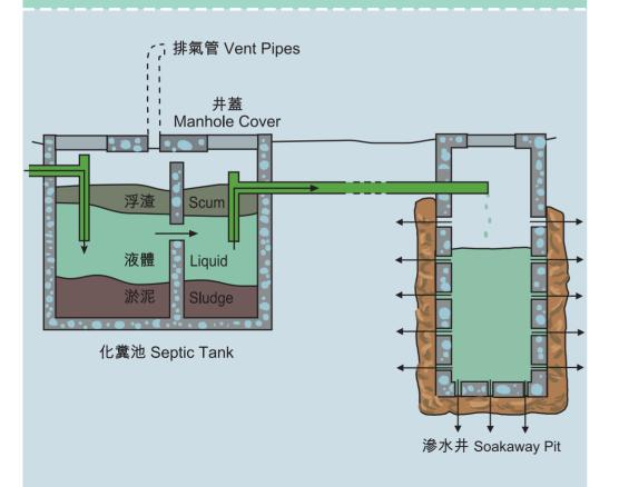
若化糞池的設計及保養不完善,蚊子便可在池內的液體滋生。要防止蚊子在化糞池內滋生,便要最少每三個月進行定期檢查一次,以確保:The liquid in the tank can provide a breeding place for mosquitoes if the tank has not been properly designed and maintained. To prevent mosquito breeding in the tank, one should inspect the tank at least quarterly to ensure that:
