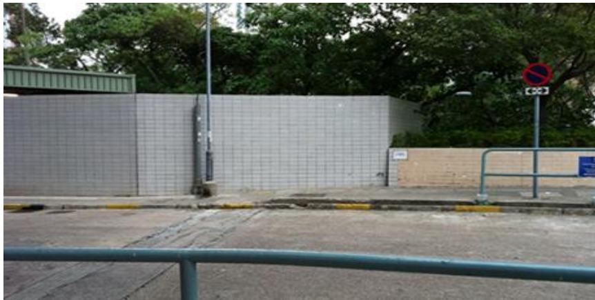
Fig.1 Proximity of flowerbed to facilities such as refuse collection point is a typical design fault in terms of rodent prevention
