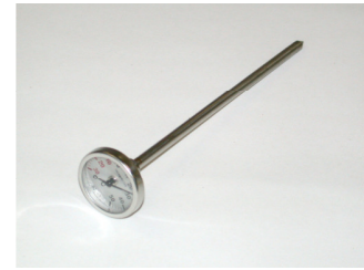
Diagram 2: Bi-metallic Stemmed Thermometer
