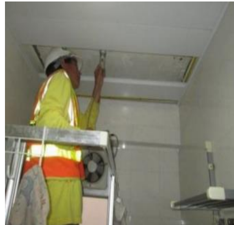
Figures 3 and 4: Consultants engaged by the JO conducting ponding test on the floor slab and using microwave tomography to detect the source of seepage.
